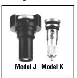
Arrow's Automatic Overnight drain operates when a compressed air system is shut down. It clears accumulated condensate from a filter bowl when pressure falls to 3 psig or less. Available for either plastic or metal bowls.
