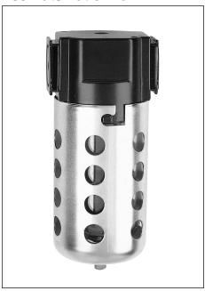
The T53 series float type drain is provided with a top threaded port. This drain features a protective stainless steel screen with an umbrella baffle, providing a large sump area for oil sludge and dirt. It is used to give continued performance and low maintenance to drain accumulated water and oil from drain lines, receiver tanks, condensate drop legs and filters.
