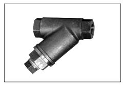
A Y Strainer installed ahead of an external drain, traps large debris and sludge; prevents malfunctions and extends the life of automatic drains.
