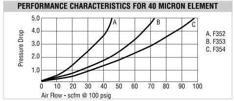
\* 5 micron element reduces flow by 10%
